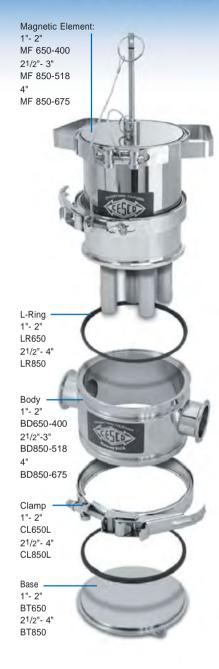
LINE CONNECTIONS: Tri-Clamp and weld ends are standard. To assure a perfect match on weld ends, specify your line's outside and inside diameters. Bevel Seat (Acme Thread), John Perry, International Dairy fittings (IDF), Q-line, I-line, pipe threads, connections with captive nuts, pipe flanges and various European sanitary ferrules are available at extra cost. Non-similar sized ends are also available. For all except our standard connections, please inquire.
